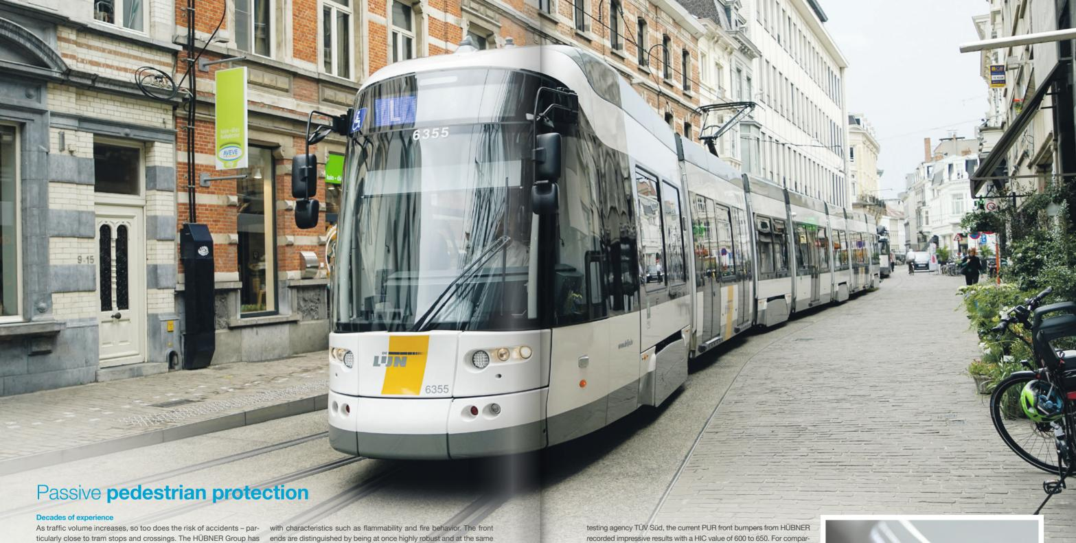
more than 30 years of experience in the production of tram front ends made of polyurethane (PUR) foam. With this expertise it is possible to combine passive pedestrian protection with modern vehicle design to best effect.
