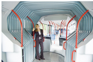
Folding bellows out of coated synthetic fabric with aluminium frames
