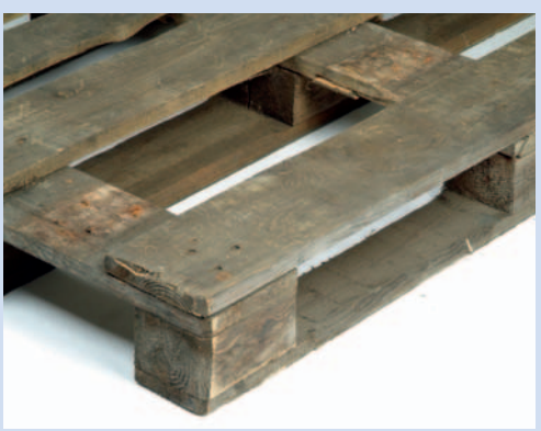
A board is missing.
