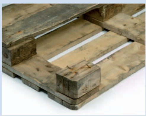
A single upper or lower leading board is damaged so that one nail or screw shank is revealed.
