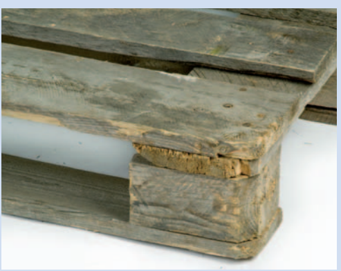
The EUR mark on the right or for example, the EPAL symbol on the left is missing.
